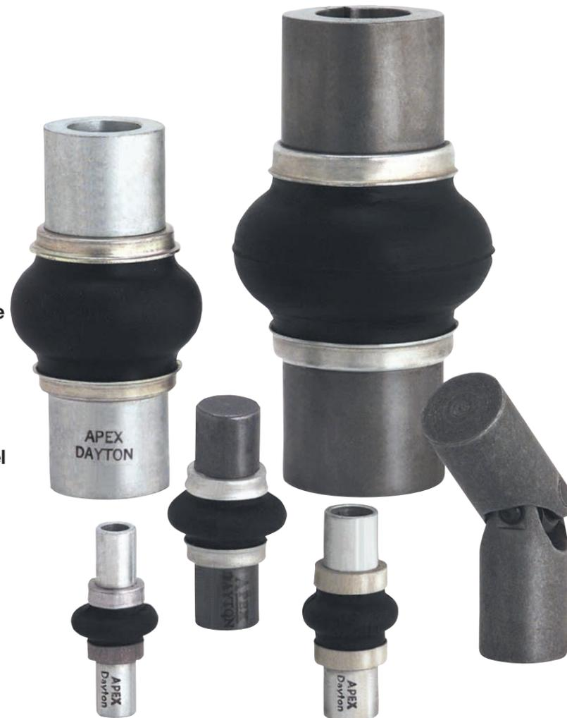
**Note:** The first number(s) after the 300 or 400 series prefix represent the outside diameter of the universal joint in 16th's of an inch. A number following this is the diameter of the bore in 16th's of an inch. If the product has a keyway it will be represented by a number following the bore size and is in 32nd's of an inch. For example, 300-20-12-6 is a 1.25" O.D. (20/16") universal joint with a .75" (12/16") bore on each end and a .188" (6/32") keyway.
