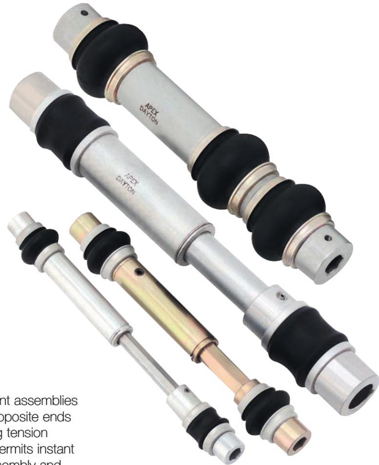
Apex Telescopic/Quick-Change universal joint assemblies consist of two universal joints mounted at opposite ends of a special spring-loaded connector. Spring tension holds the assembly in driving position, yet permits instant removal by compressing one end of the assembly and lifting it clear.
